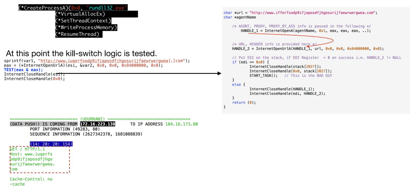
If this connection is successful, executable won't follow the code path for destruction. Kill switch is normally used to evade sandboxing OR **stop the infection by spawning the domain.**
